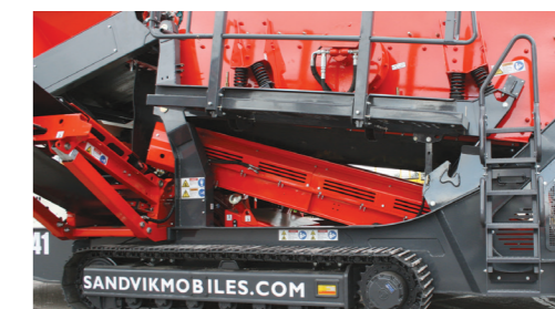
Screen box jack up facility allows easy access
