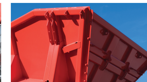
Split rear hopper door for direct feeding
