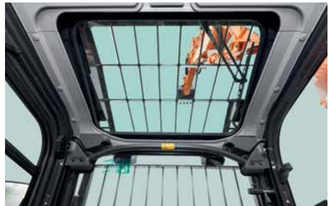
Roof window with wiper enhances visibility.
