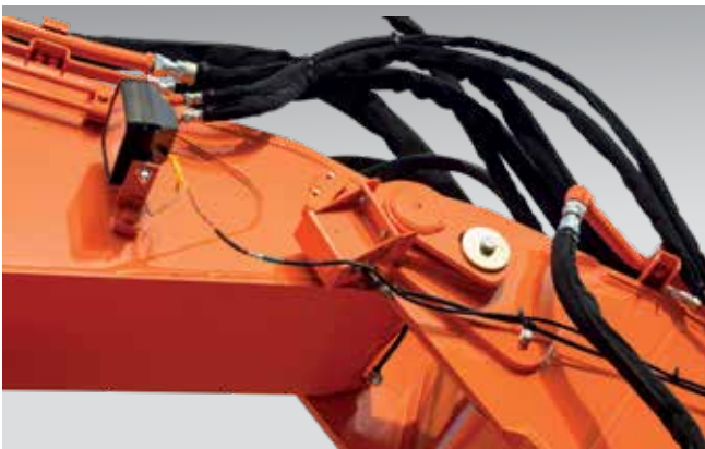
Working range warning device for safe operation.
