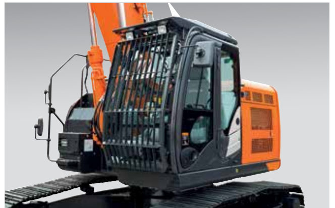
The cab's front and top guard (OPG level 2) provides added protection.
