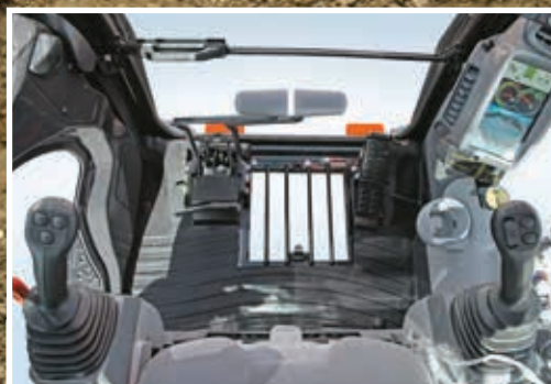
A window in the floor of the cab gives a better view of the site below.
