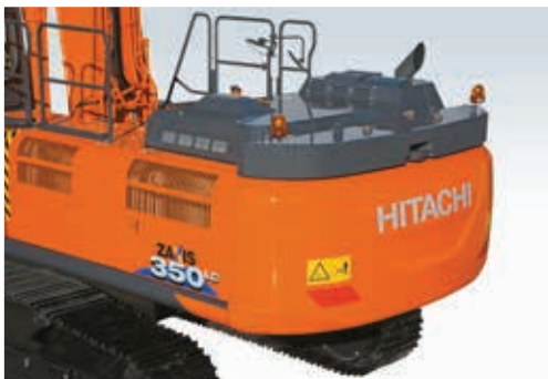
The detachable counterweight enhances the machine's versatility.
