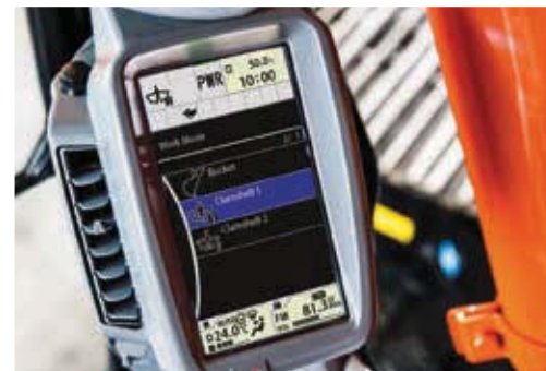
Switch between workmodes via the monitor.
