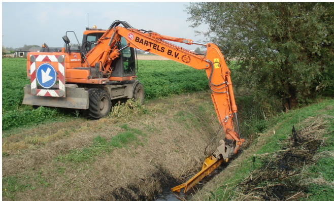
The Herder mowing bucket can be attached directly to the excavator.
