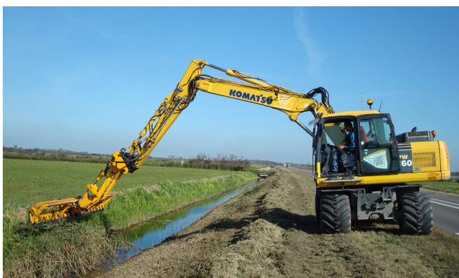
An excavator with the mowing bucket on an extension piece for extra reach.
