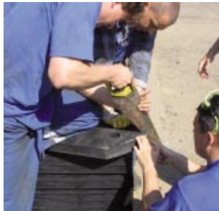
Sandvik WT7000 dual hardness modular wear plates can easily be cut on site using a hand saw.
