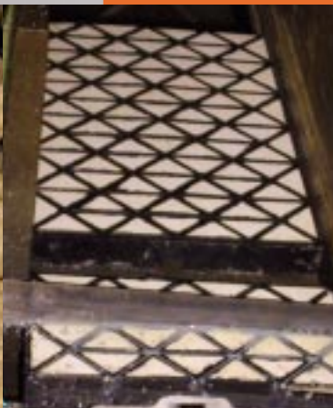
The triangular shaped tiles make it easy to cut the ceramic wear plates to fit the application.
