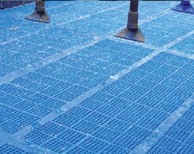
Tensioned PU screening media
