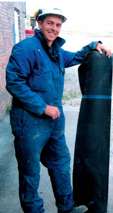
Tensioned rubber screening media
