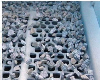
Tensioned rubber screening media
