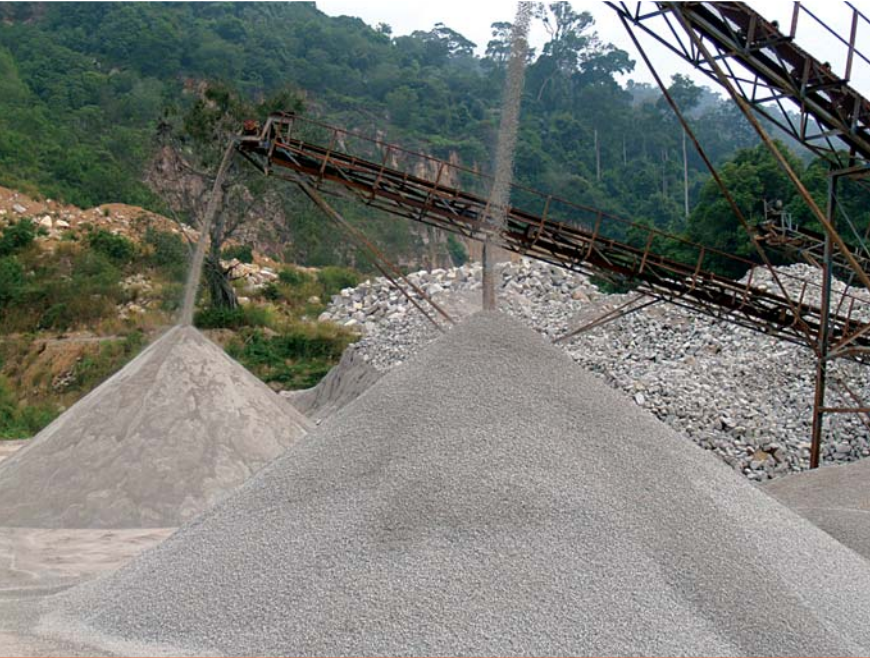
Quality manufactured sand 0-5 mm and premium shaped aggregate 5-10 mm.
