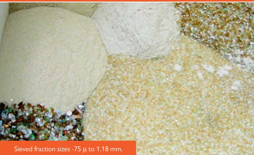
Quality manufactured sand 0-5 mm and premium shaped aggregate 5-10 mm.
