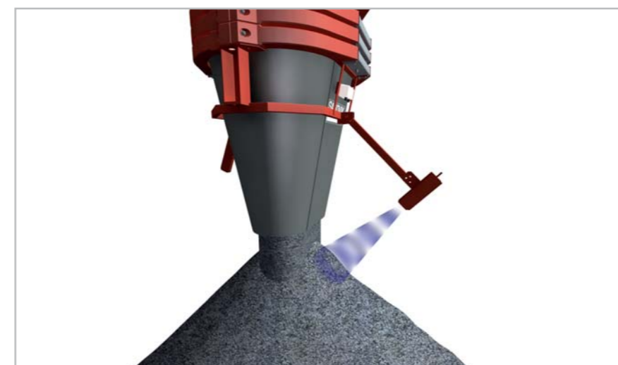
The automatic level sensor means that the Sandvik WE8000i telescopic chute senses its height above the stockpile, and adjusts it so that the risk of dust emission is always minimized.
