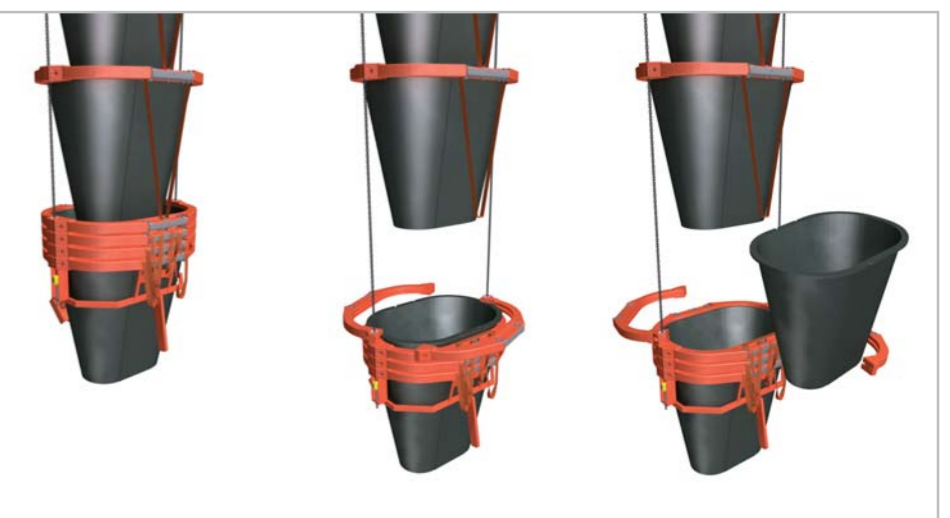
The carrying collar can be separated easily, and the chute segment replaced or turned. The modular design reduces down time and spare parts costs.
