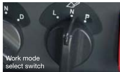
P mode: Heavy-duty excavation N mode: Loading L mode: Light-duty operation
